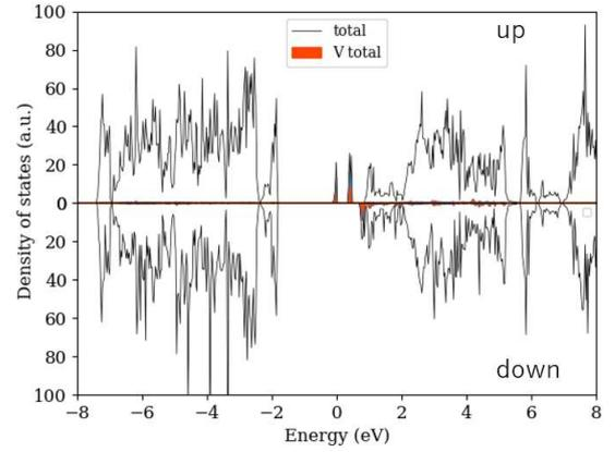
**Fig. 4** DOS of V-doped  $\text{Bi}_2\text{Zr}_2\text{O}_7$  supercell.
