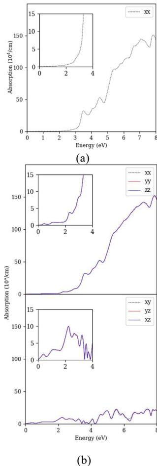
**Fig. 7** Absorption coefficient,  $I$ , for the (a)  $\text{Bi}_2\text{Zr}_2\text{O}_7$  unit cell and (b) V-doped  $\text{Bi}_2\text{Zr}_2\text{O}_7$  supercell.
