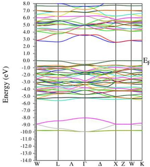
**Fig. 2** Energy band structure of  $\text{Bi}_2\text{Zr}_2\text{O}_7$ .
