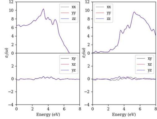
**Fig. 6**  $\varepsilon_1(\omega)$  and  $\varepsilon_2(\omega)$  of the theoretical dielectric function of the V-doped  $\text{Bi}_2\text{Zr}_2\text{O}_7$  supercell.
