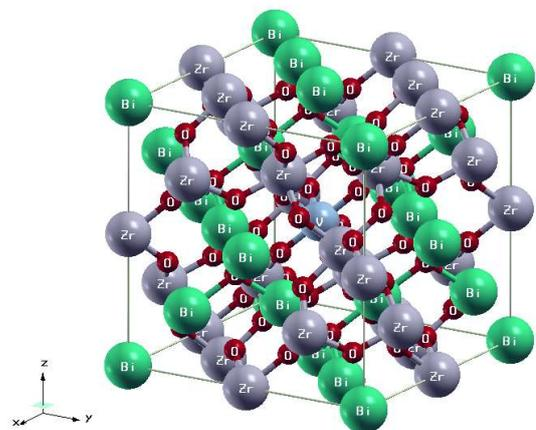
**Fig. 1** V-doped Bi<sub>2</sub>Zr<sub>2</sub>O<sub>7</sub> supercell.
